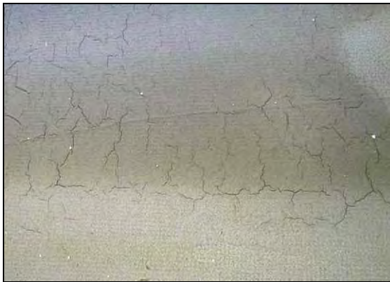
Base Coat Applied Too Thickly
