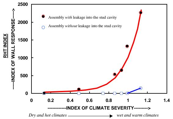
Example of the predicted RHT response of a given wall assembly with and without leakage into the stud cavity (i.e. with and without deficiencies), as a function of the climate severity. The more severe the climate (the higher the value of the index on the X axis), the higher the "RHT" response (Y axis) for the wall with water leakage into the stud cavity.
